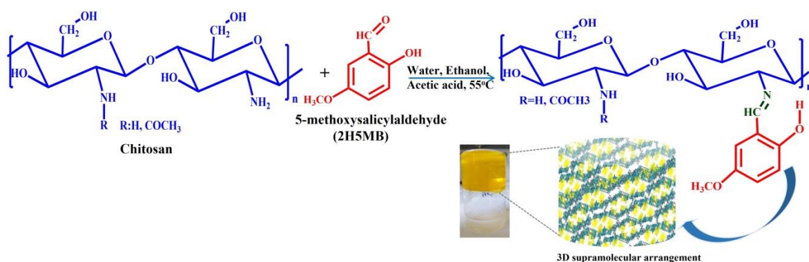
Figure 1. Synthesis of chitosan-based hydrogel.
